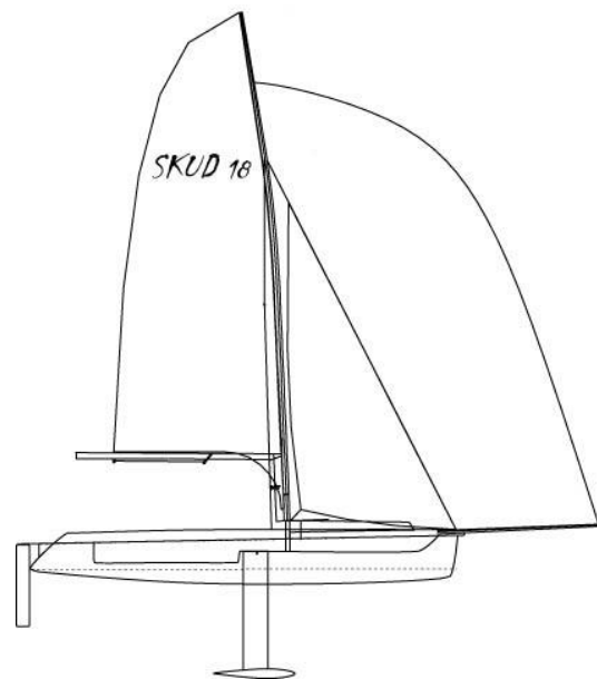
SKUD 18 5.8m Sloop Rigged Two Person Self Tacking Jib Asymmetric Gennaker Twin Rudder Blades
