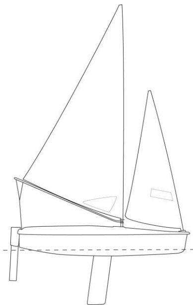
Liberty 3.6m Schooner Rigged Single Person Self Tacking Jib with Strut Twin Rudder Blades
