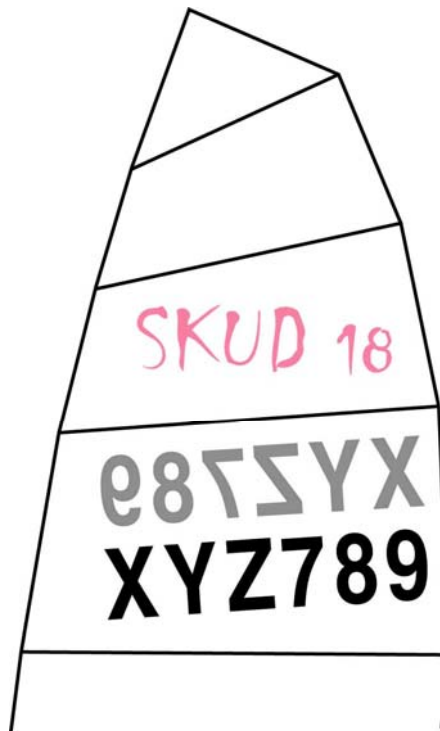
SKUD 18 Insignia - Hot Pink Pantone 812U Insignia reads correctly from Port side
